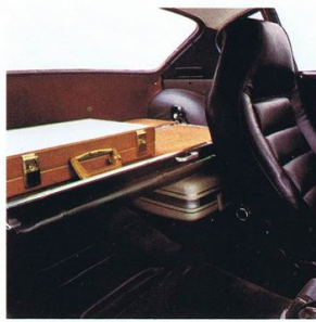
The rear seat backrest can be dropped to provide a flat surface for storing extra luggage. Which can then be strapped down.
