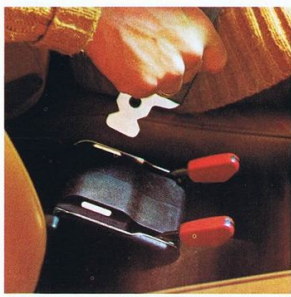
Front seat belt locks have their own light so you can find them at night. If the driver doesn't buckle his belt a warning lamp on the dash will remind him to . . . day and night.
